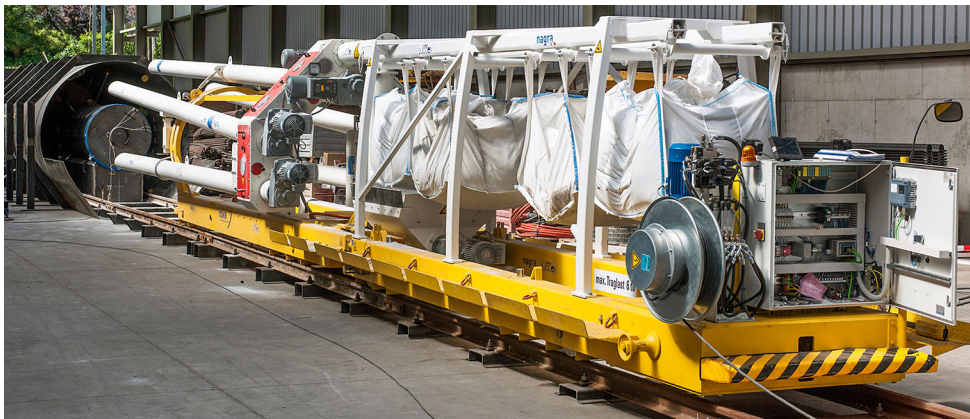
Fig. 16 Photo (by COMET) of the prototype BFM (with the control unit at the back and the feeding unit carrying four bigbags) during the mock-up backfilling test at a workshop in Grono, Switzerland
