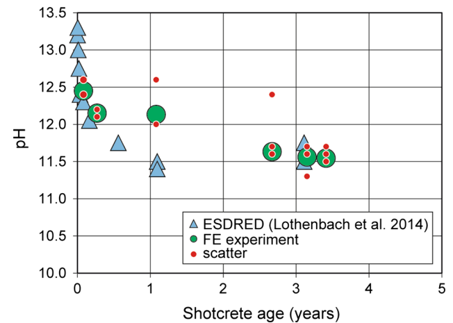
Fig. 7 The filled green circles show the pH values of FE samples measured under laboratory conditions at different shotcrete ages. The small red circles are all individual measurements. The values for the ‘ESDRED mixture’ as described in Lothenbach et al. (2014) are represented by blue triangles
