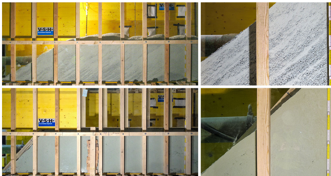
Fig. 14 ‘Fir-tree like’ segregation effects due to small material avalanches at the slope as seen in the second pre-test ( top pictures ) can easily be avoided by covering the slope, e.g. with a flexible mat ( bottom pictures )
