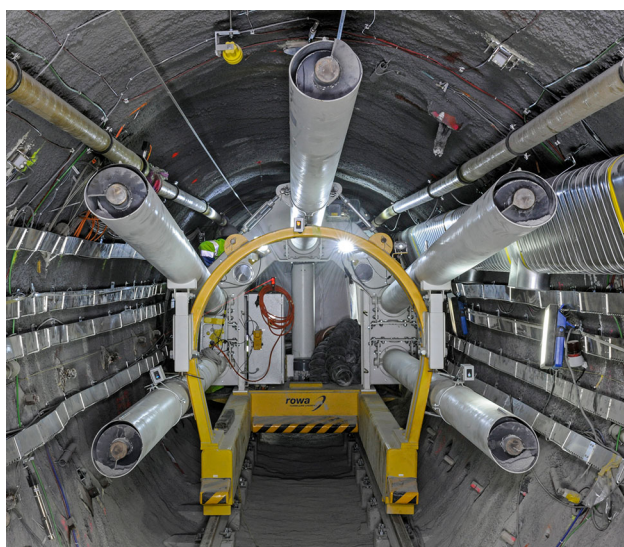
Fig. 19 Photo (by COMET) of the prototype BFM in the FE tunnel at the Mont Terri rock laboratory
