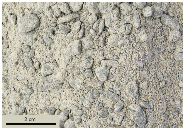
Fig. 13 Photo of the highly compacted ‘granulated bentonite mixture’ (GBM) produced for the FE experiment. For the individual pellets, an average dry density of 2.18 g/cm 3 was achieved by compaction between flat rollers
