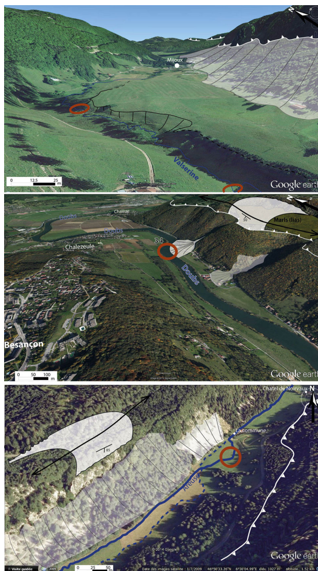
Fig. 7 Field observations along flow paths of the Valserine, Doubs and Areuse rivers (see Fig. 4 for locations). a Valserine valley path in the High Range of the Jura Mountains. The NE–SW directed thrust created a topographic relief, which results in several landslides and rockslides. This valley was filled by glacial deposits and the river incision created a step involving frequent landslides which are correlated with knickpoint location (red circles). b The Doubs River upstream Besançon (External Range). The ENE–WSW directed thrust combined with erosion of the anticline hinge created landslides and rockslides. The younger one (in white) is correlated with knickpoint location (red circle, knickpoint 34 on Fig. 6). c The Areuse steep sided valley trough the High Range. This valley corresponds to a remnant syncline between two NE–SW directed tight folds. The southeastern most one is over-thrusted on the syncline decreasing the valley width. The anticline on left side of the river has a very steep southwestern flank involving frequent landslides and rockslides. On this picture at least two rockslides can be determined; an old one (in transparent light grey) already covered by a forest and a younger one (in transparent white) not yet covered by vegetation. It is still possible to see the ancient river path (in blue dot line). The river has presently restored its path following the older landsliding disturbance but remains deviated by the more recent one, which corresponds to a knickpoint location (red circle)
