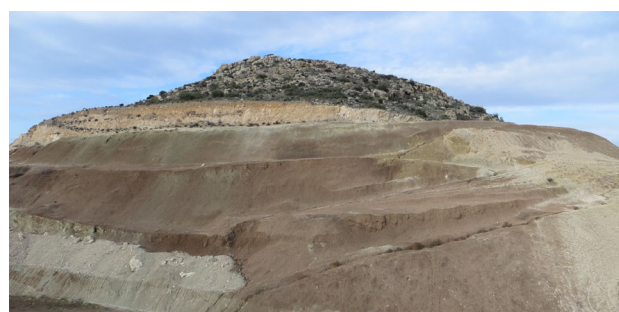
Fig. 2 Bentonite quarry near Kato Moni, Cyprus. Bentonite (greenish/reddish) is overlain by limestone cap rock and colluvium deposits
