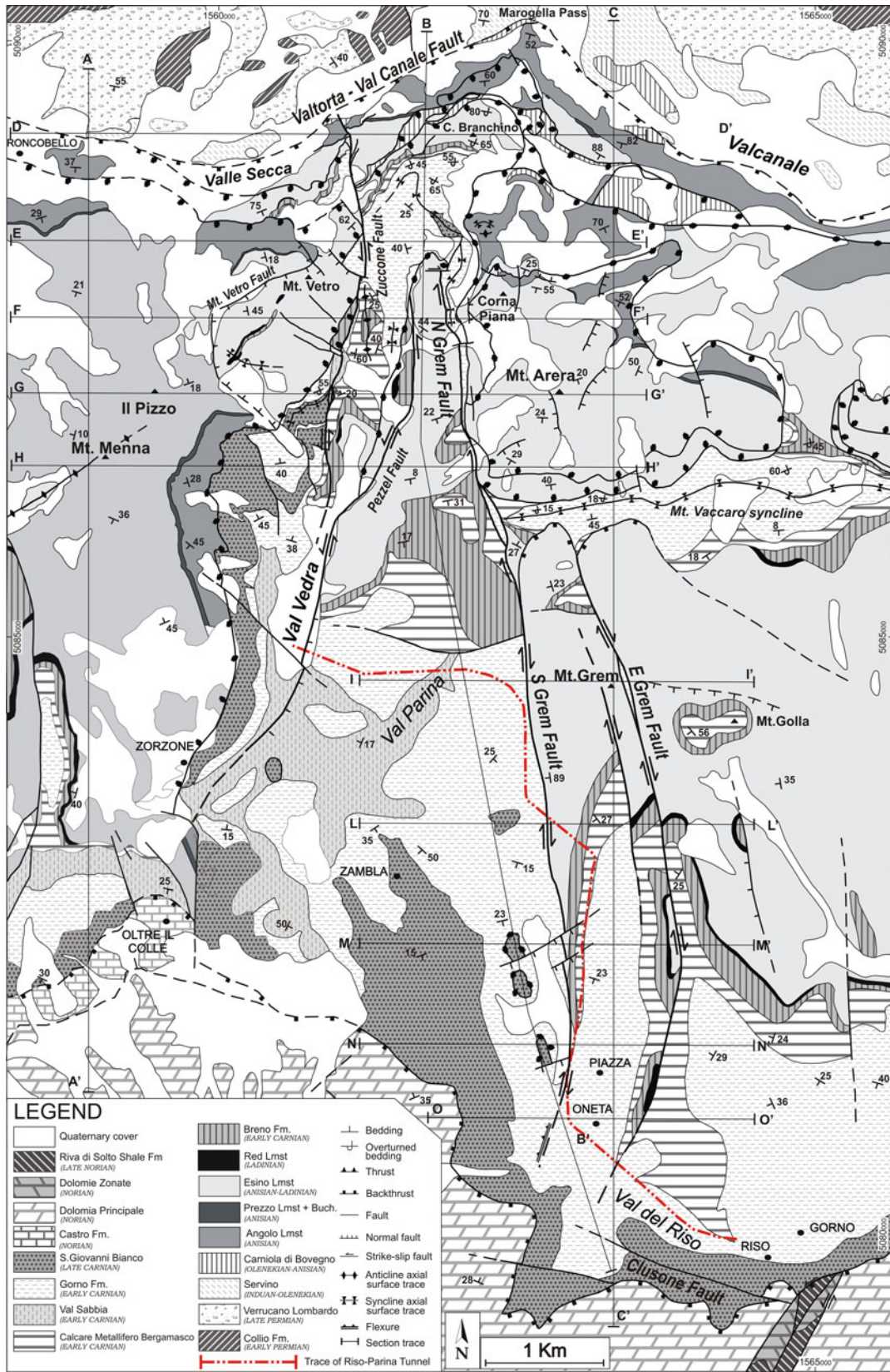
Fig. 2 Geological-structural map of the GVTZ from original field mapping at 1:5,000 and 1:10,000 scale. Key to fault nomenclature (applies to all succeeding figures): N Grem fault, northern segment of
