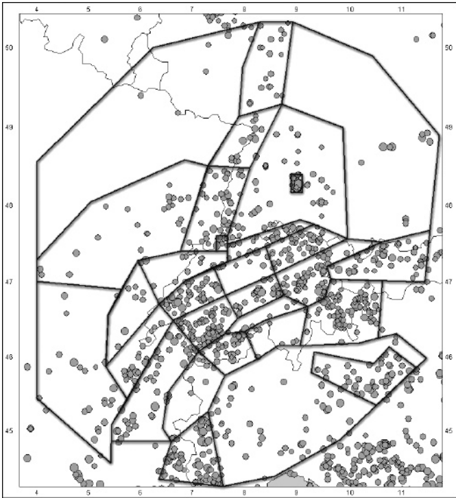
Fig. 3. The basic zone model of EG1c; shown also is the seismicity \geq 3.5 Mw since 1750.
