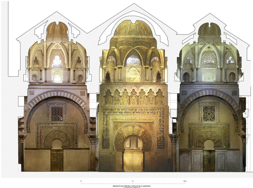
Fig. 11 Section of the domes over the maqsura in the Great Mosque of Cordova. Image: Photogrammetric survey by Antonio Almagro
