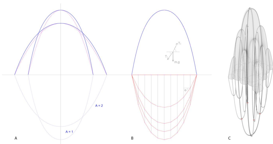
Fig. 3 A Catenary curves in blue, parabolas in magenta, B particles are equidistant at rest position at the start of the simulation, C particle-spring system simulating hanging chains
