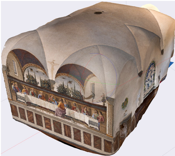
Fig. 4 San Marco's refectory: 3D model of the room with scaled painting mapped on the model. Image: authors
