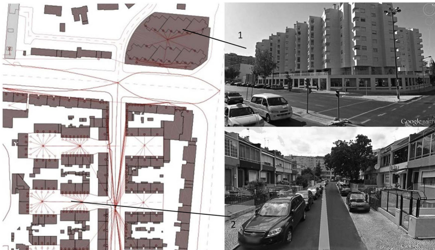
Fig. 1 1 Av.EUA: detail of building standing on a plateau; 2 row houses at R. Guilhermina Suggia. Some of the commercial spaces in the plateau were never used. The entrances to the distribution hall of the apartment buildings face the elevated backyard in the plateau. The long thin building in the upper left corner has all entrances facing the back street
