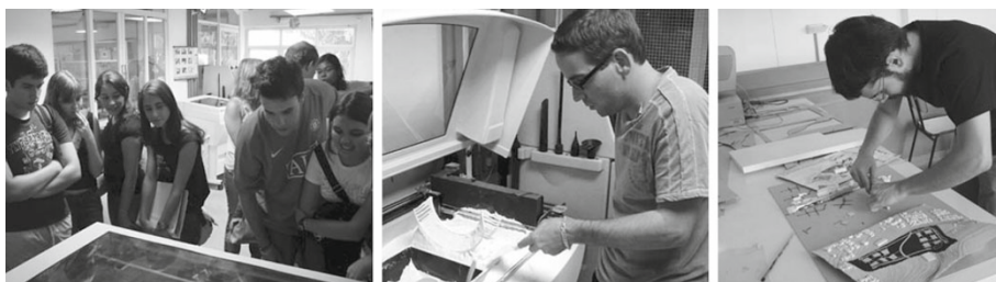
Fig. 3. Digital fabrication lab: students gather around the laser cutter; removing a model from the 3D printer; assembling a model with rapid-prototyped parts
