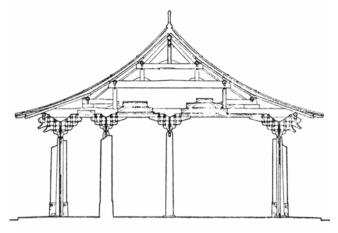
Fig. 5. The Sanqing dian of Yongle gong (1262), with columns located between purlins [Du 1963]
