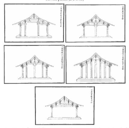
Fig. 6, a–e. New 6-rafter *ting* hall sections generated by our grammar (redrawn in the style of the *Yingzao fashi*)
