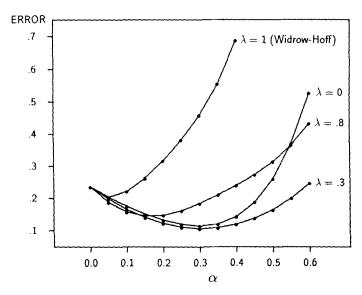
Figure 4. Average error on random walk problem after experiencing 10 sequences. All data are from  $TD(\lambda)$  with different values of  $\alpha$  and  $\lambda$ . The dependent measure is the RMS error between the ideal predictions and those found by the learning procedure after a single presentation of a training set. This measure was averaged over 100 training sets. The  $\lambda=1$  data points represent performances of the Widrow-Hoff supervised-learning procedure.
