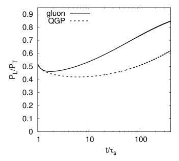
Figure 1. Time evolution of the pressure ratio  $\mathcal{P}_L/\mathcal{P}_T$  obtained from the numerical solution of the Boltzmann equation in the small angle approximation, for a pure gluon system (solid line) and a quark-gluon plasma (QGP, dotted line). Here  $\tau_s$  is a natural microscopic time scale, proportional to the inverse of the saturation momentum  $Q_s$  (see section 3.2 for details).
