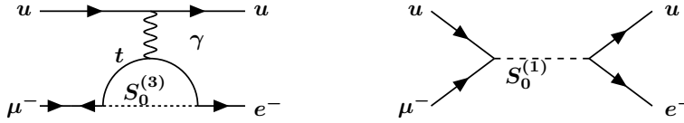
Figure 2. Loop and tree leptoquark contributions to \mu N \rightarrow e N' . The diagram represents leptoquarks with quark flavour (= generation number), as considered in section 4. For the various patterns of \lambda 's that we consider, the loop diagram involving third generation quarks dominates.
