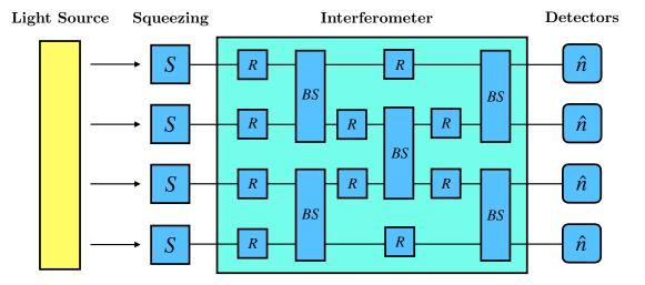
**Figure 5.** A Gaussian boson sampling device. It consists of a set of squeezing gates, an interferometer and photon detectors. The interferometer itself is constructed from rotation gates and beamsplitters.
