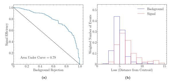
**Figure 6.** (a) shows the ROC curve for K-means anomaly detection method trained on feature vectors constructed from GBS samples. The distribution of the loss for the signal and background test sets is shown in (b).
