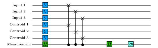
Figure 7. Diagram of the Q-means quantum circuit. The feature vector and centroid is encoded through  $U_3$  gates, while a SwapTest is used to provide a measure of their similarity.
