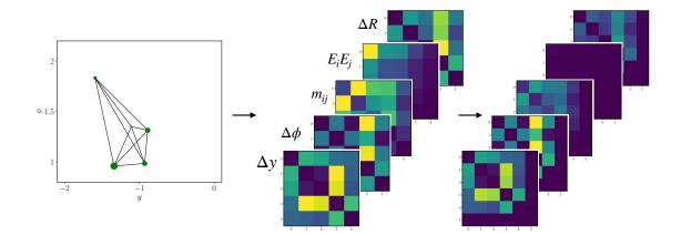
**Figure 3.** For a graph we find five weighted adjacency matrices from it, each one capturing features of the graph nodes. These five are then scaled and padded, giving the final matrices on the right. These can be embedded and used as input to classification algorithms.
