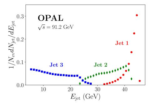
Figure 18. OPAL results for the energy spectrum of the leading jet (Jet 1) and the first two subleading jets (Jet 2,3) using 3-jet events. Data taken from [142].
