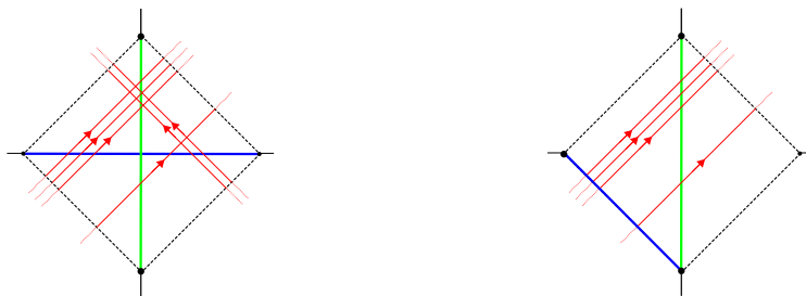
Figure 5. Left: in a CFT, one can change a spatial interval (blue) into a time interval (green) using null paths, preserving information flow. Right: in a chiral (sector of a) CFT, one can move the endpoint of the interval (blue) along one of the null directions, e.g. up to the time interval (green), and preserve the information flow.
