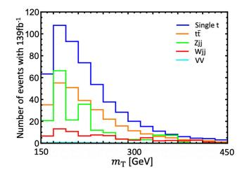
Figure 2. Expected SM BG  $m_{\rm T}$  distributions after applying all kinematic cuts, shown as number of events per  $m_{\rm T}$  bin. We assumed 139 fb<sup>-1</sup> of data. The colors distinguish the different BG categories, as detailed in the upper right corner.
