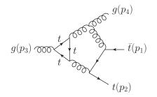
Figure 7. Feynman diagram contributing to  $A^{(2),N_h}$  that leads to the new master integral topologies shown in figure 6. The solid lines denoted the top quark whereas spiral lines denote the gluons. All external momenta are on-shell.
