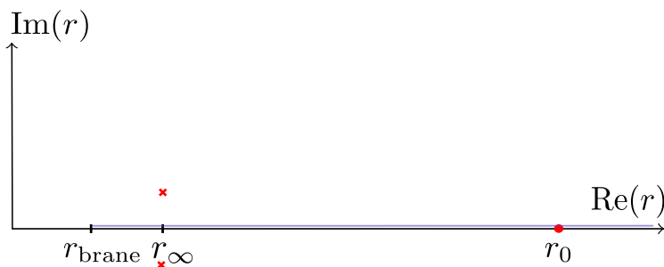
Figure 15. Integration contour for eq. (B.49), spanning from r_{\text{brane}} to \infty . The figure highlights the positions of significant features within the contour. The two branch points of the integrand are marked by red crosses, situated at r_\infty \pm i\frac{L^2}{2r_\infty}\delta P . The red dot represents the pole of the integrand located at r_0 . Deep in this region of parameter space, r_\infty - r_{\text{brane}} \gg \mathcal{O}(\delta P) .
