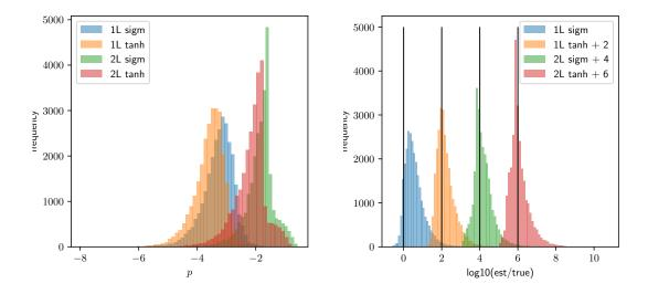
**Figure 3**. Left: number of digit accuracy for the two integrals for two different activation functions. Right: ratio of the actual error of the standard deviation of the replica results. The histograms are shifted for readability. The vertical lines correspond to the actual error matching the standard deviation of the network predictions.
