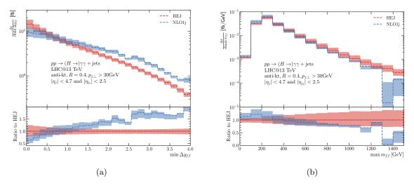
Figure 7. High-energy sensitive inclusive 1-jet distributions: (a) the minimum rapidity separation between any two outgoing particles (Higgs boson or jets) and (b) the maximum invariant mass between any two outgoing particles (Higgs or jets). HEJ results are rescaled by the inclusive cross section ratio  $\sigma_{\rm NLO1J}/\sigma_{\rm HEJ \ IJ}$ .
