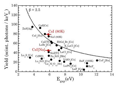
Figure 4. Light yield of scintillators and phosphors as a function of bandgap, adapted from [68]. A dotted line indicates a model-dependent maximum light yield [68]. Red dots mark our measurements for cryogenic CsI, in agreement with [63, 65], and for room temperature CsI[Na] [4]. Yields of up to 125 ph/keV<sub>ee</sub> have been claimed for other CsI stock [59, 60]. A CsI bandgap range is indicated by horizontal error bars [70].
