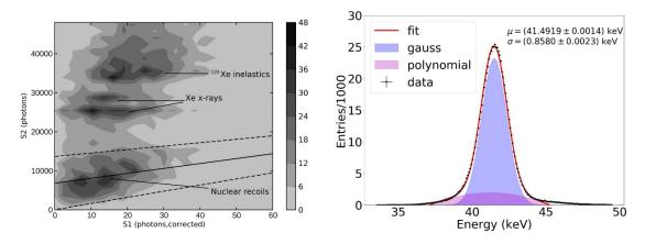
**Figure 9.** Left: nuclear recoil identification in a gaseous xenon detector by using S1/S2 discrimination [104]. Right: example of energy resolution obtained for 41.5 keV gammas [105]. The very small Fano factor in xenon gas, two orders of magnitude lower than for liquid xenon, allows for excellent energy resolution even in large-scale detectors [106].
