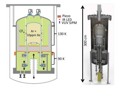
**Figure 11**. Schematic and model of a 10-kg LAr bubble chamber under construction, showing pressure and temperature control, bubble imaging, and scintillation detection scheme. The design is of a "right side up" type, as in [123] and the upcoming PICO-40 and PICO-500 chambers at SNOLAB. Rendering by Fermilab's PPD/Mechanical Engineering Department.
