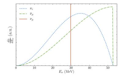
Figure 2. Neutrino flux spectra expected from pion DAR, in arbitrary units (a.u.), as a function of the neutrino energy in MeV. The three components of the flux are shown separately as indicated by the legend. The distributions have been normalized to one.
