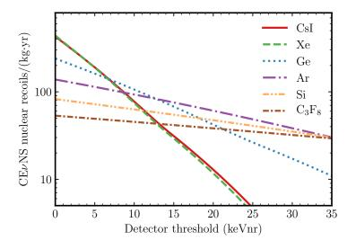
Figure 7. Expected integrated  $CE\nu NS$  rate above nuclear recoil threshold, 20 m away from the ESS target, for all detector materials considered in this work. All technologies considered for use at the ESS have thresholds at or below 1 keV<sub>nr</sub>.
