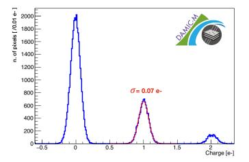
Figure 8. (From [94]) First demonstration of single-electron sensitivity in DAMIC-M CCDs, using a Skipper readout. An average ionization energy deposition of 3.77 eV is necessary for the creation of a  $1 e^{-1}$  signal in silicon [95].
