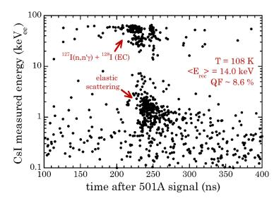
Figure 5. First measurement of nuclear recoil quenching factor (QF) for cryogenic CsI. The figure displays the measured electron-equivalent energy (keV<sub>ee</sub>) deposited by 14 keV Cs and I nuclear recoils induced by 2.2 MeV neutron scattering. The reader is referred to a similar figure 2 in [71], for more details on the methodology employed in QF determination.
