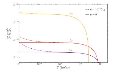
Figure 15. Differential cross section for  $CE\nu NS$ , as a function of the recoiling energy of the nucleus, in the SM and in presence of a non-vanishing neutrino magnetic moment  $\mu = 10^{-10}\mu_B$ . The different colors correspond to different target nuclei, as indicated by the labels. The incident neutrino energy is set to  $E_{\nu} = 40 \text{ MeV}$  in all cases, and the cross section in the SM ( $\mu = 0$ ) is also shown for comparison.
