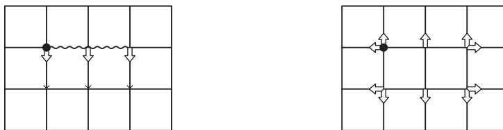
Figure 8. Each link of the graph is associated with an holonomy and the thick arrow represents the corresponding conjugated flux. The black dot represents the root at which gauge invariance is relaxed. The left panel shows an example of construction of a coarser flux. Fluxes are first parallel transported to the root following the path defined by the wiggly line and then added to form a coarser flux. The right panel shows an example of closed path. As before, fluxes must be first parallel-transported to a common frame before being added to each other. In presence of curvature, this sum will not be zero meaning that the Gauß constraint is violated.
