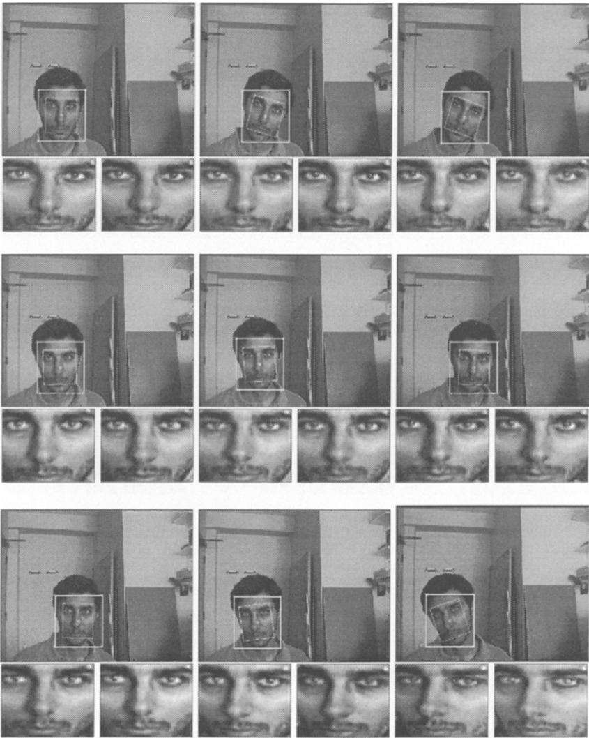
Fig. 9. Every 10th frame from a sequence with attentional windows and aligned face images overlaid. Below each frame are the located region (left) and its reconstruction (right). The affine parameters were recovered using LES.
