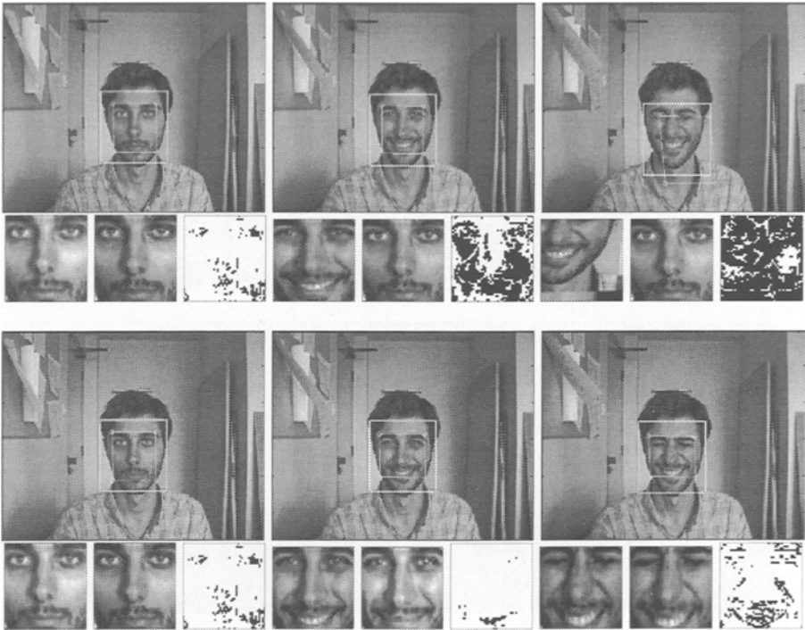
Fig. 8. This sequence demonstrates the advantage in using shape with non-rigid expression changes. The first two frames show the overlaid results from EigenTracking without shape. The corresponding three small images are, from left to right, the aligned object image, the reconstructed object image using the estimated affine parameters, and the outliers. The last two frames show the results on the same sequence from the adaptive scheme with shape encoded.
