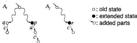
Fig. 4. critical extension which might lead to a deadlock
