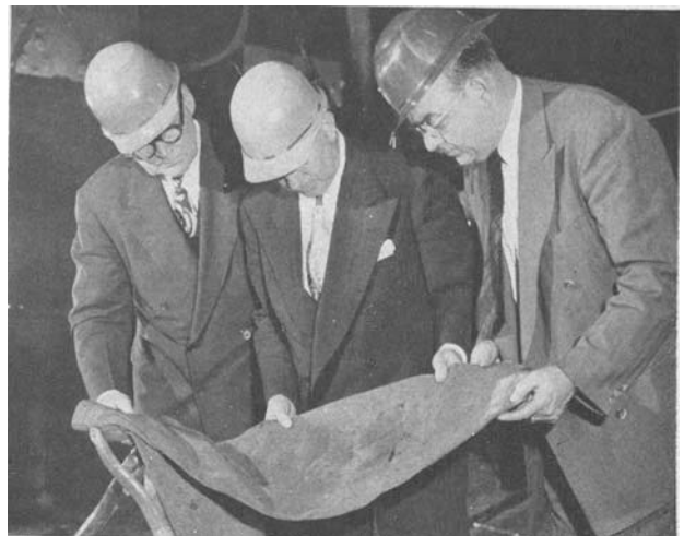
Fig. 1— These flameproofed trousers were subjected to several severe washings with the most caustic materials and then completely dried before the test was made. After the ladle containing liquid metal at 2800°F from the open hearth was emptied there was no flame or glow (Left).
