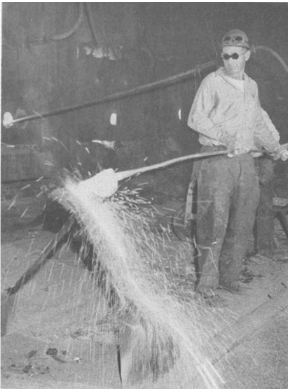
Fig. 1— These flameproofed trousers were subjected to several severe washings with the most caustic materials and then completely dried before the test was made. After the ladle containing liquid metal at 2800°F from the open hearth was emptied there was no flame or glow (Left).
