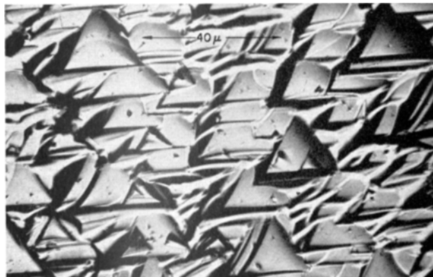
Fig. 1—WAg etched germanium surface. Approximately (111) orientation.
