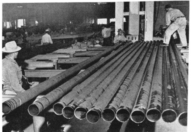
Metallurgists inspect the first seamless tubing turned out by the new CF&I mill at Pueblo, Colo. Primary market aim for the mill is gas and oil producers in the western U. S. and Canada area.
