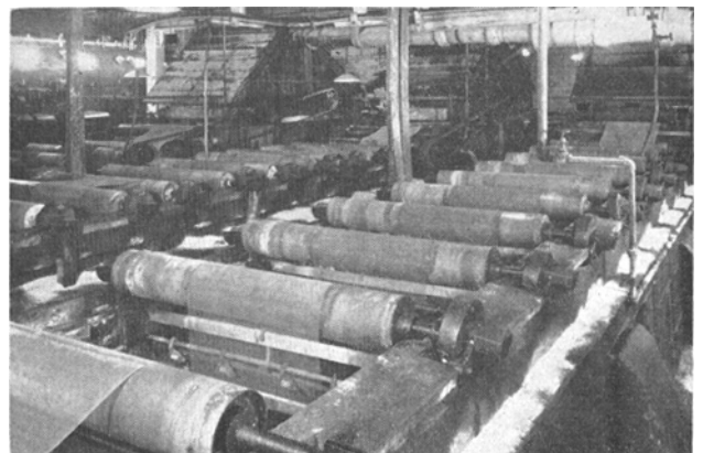
Three galvanizing tanks can be seen from this end of the galvanizing dept. Total number of tanks in operation is six.
