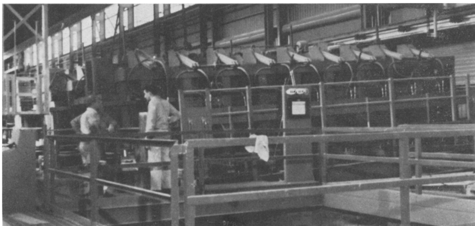
Controlled Pressure Pouring of stainless steel slabs is the feature of Washington Steel Corp.'s new melt shop near Washington, Pa. Soon to be on stream, it will be the first fully commercial unit of its kind. Above and below are shown the graphite slab molds.
