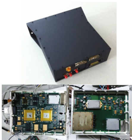
Figure 1 HiSGR receiver and internal components
