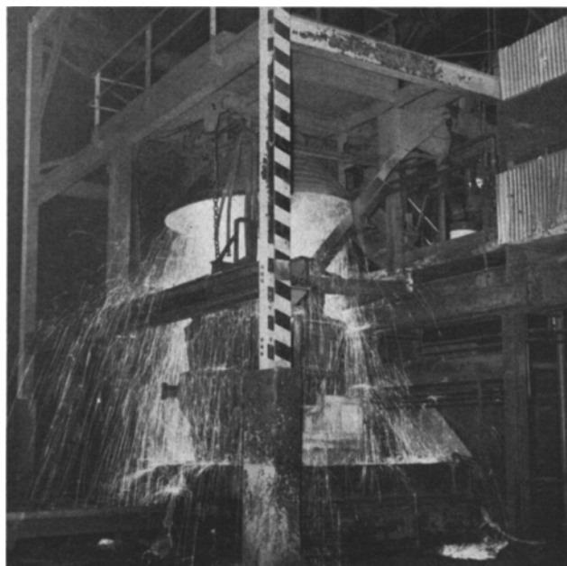
Oxygen refining ferrochrome at the Marietta, Ohio, plant of Union Carbide Metals Co.
