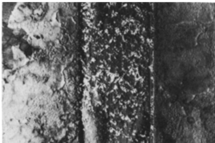
Fig. 2 (left)—A \frac{1}{4} \times \frac{1}{2} -in. flaw on a coated Cb tab after reheating to 1800°F in air for 20 hr. X3.
