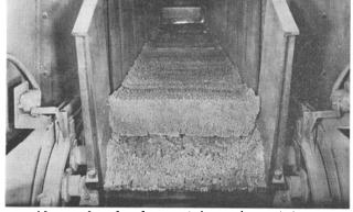
Also under development is equipment to use the up-draft principle of sintering. The sintering strand pictured at right is equipped for such experimentation.
