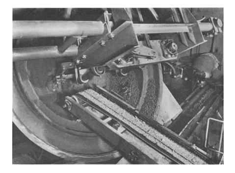
Currently under development is a disk agglomerator, or *flying saucer*, for agglomerating fines into a uniformly sized pellet for use in sintering. As the flying saucer revolves, the fines fed into the innermost saucer agglomerate. With increasing particle size, the pellets tumble over successive lips to the outer ring where they pass over the last lip and on to further processing.
