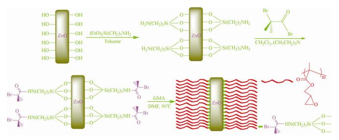
Scheme 1. Surface functionalization of ZnO Nanowires and polymerization of the initiator-functionalized wires.
