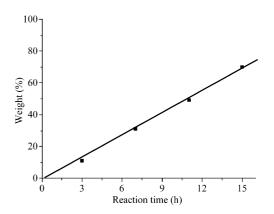
FIG. 5. The effect of the polymerizing time on the polymer weight values.
