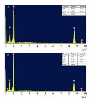
FIG. 2. Energy dispersive X-ray spectroscope of (A) ZnO nanowires; (B) PGMA-ZnO nanowires.
