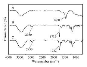
FIG. 3. IR spectra of (A) ZnO-NH<sub>2</sub> nanowires; (B) PGMA-ZnO nanowires; (C) after treatment of PGMA-ZnO nanowires in HCl solution.
