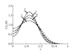
FIG. 2. Calculated distribution of dopant after annealing with continuance  $\Theta = 0.0025D_{0l}/L^2$  (curves 1 and 3) and  $\Theta = 0.005D_{0l}/L^2$  (curves 2 and 4). Curves 1 and 2 are corresponding to spatial of distribution of dopant in homogeneous material. Curves 3 and 4 are correspond to spatial distribution of dopant in *SH* for  $D_{1l}/D_{2l}$ =4. Solid lines are analytical results. Dashed lines are numerical results. Coordinate of interface is equal to a=L/2.
