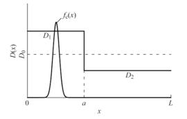
FIG. 1. Semiconductor heterostructure, which consist of an epitaxial layer  $(x \in [0,a])$  and a substrate  $(x \in [a,L])$ .
