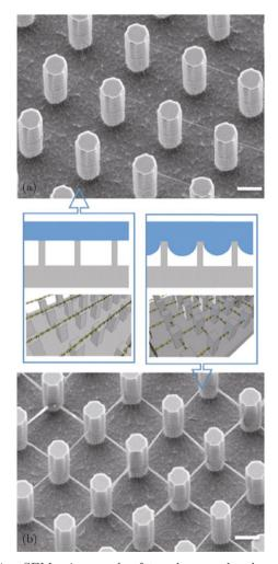
Fig. 4 SEM micrograph of two large ordered arrays of stretched DNA bundles. These arrays are obtained before (Panel a) and after (Panel b) the occurrence of the Cassieto-Wenzel transition. The scale bar corresponds to a length of 5  $\mu$ m. The ordered array shown in panel b has been acquired in the square-shaped region highlighted in Fig. 2(b).
