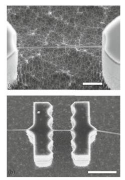
Fig. 1 SEM micrographs show suspended DNA bundles on a square shaped pillar (panel a) and a saw-shaped pillar (Panel b). In both cases DNA bundles are precisely pinned to structural features resembling tips. The scale bar corresponds to a length of 2  $\mu$ m (Panel a) and 5  $\mu$ m (Panel b).
