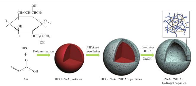
Fig. 1 Schematic representation of the preparation of PAA-PNIPAm hydrogel capsules.
