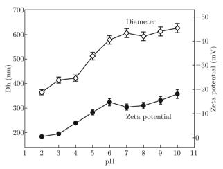
Fig. 6 Size and zeta potential of PAA-PNIPAm hydrogel capsules at different pH.
