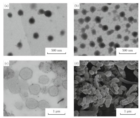
Fig. 2 TEM images of (a) HPC-PAA particles (pH = 2.4); (b) HPC-PAA-PNIPAm composite particles (pH = 2.4); and (c) PAA-PNIPAm hydrogel capsules (pH = 8.0). (d) SEM image of PAA-PNIPAm hydrogel capsules after frozen drying treatment.
