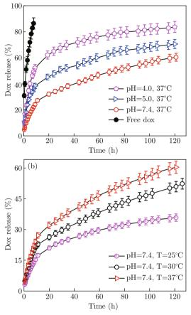
Fig. 5 Release profiles of Dox from the hydrogel capsules in PBS with different (a) pH and (b) temperatures.
