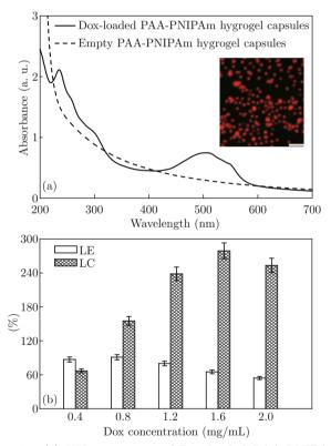
Fig. 4 (a) UV-vis spectra of Dox-loaded PAA-PNIPAm hydrogel capsules and empty PAA-PNIPAm hydrogel capsules; (inset) the LCSM image of the Dox-loaded PAA-PNIPAm hydrogel capsules, the scale bar is 2  $\mu$ m; (b) LC and LE of PAA-PNIPAm hydrogel capsules corresponding to different feeding Dox concentrations at pH = 7.0.
