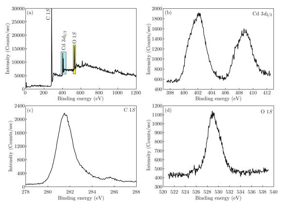
Fig. 3 XPS results for the prepared Cd-doped Co/C NPs. (a) The whole survey; (b), (c) and (d) are the low scan rate investigations for Cd  $3d_{3/2}$ , C 1S and O 1S orbits, respectively.
