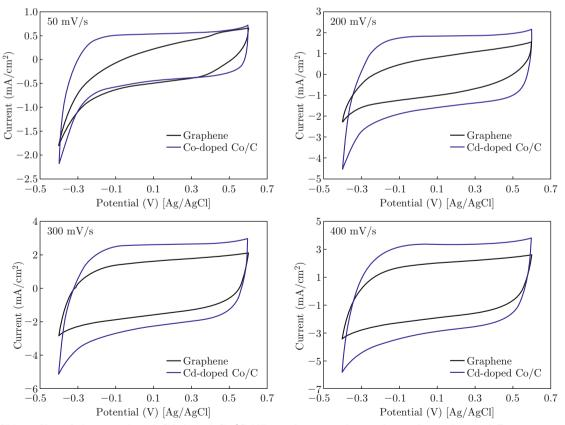
Fig. 10  $\,$  CV profiles of the introduced Cd-doped Co/C NPs and prepared greaphene electrodes at different scan rates and NaCl concentration of 0.1 M.
