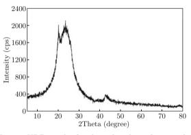
Fig. 6 XRD results for the reduced graphene oxide.
