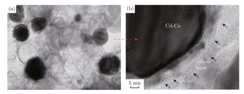
Fig. 4 TEM (a) and HRTEM (b) images for the prepared Cd-doped Co/C NPs. The arrows clarify the carbon layer enveloping.
