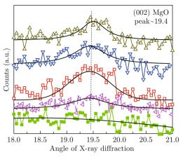
Fig. 3 X-ray diffraction scan curves of MgO films. Solid lines are fitting curves. The deposition conditions of MgO film: ( $\square$ ) RF power 170 W, Ar pressure 12 mTorr, separation distance 5 cm; ( $\blacksquare$ ) 170 W, 12 mTorr and 9.5 cm; ( $\triangledown$ ) 170 W, 5 mTorr and 5 cm; ( $\triangle$ ) 170 W, 8 mTorr and 5 cm; ( $\triangle$ ) 170 W, 12 mTorr and 6 cm.
