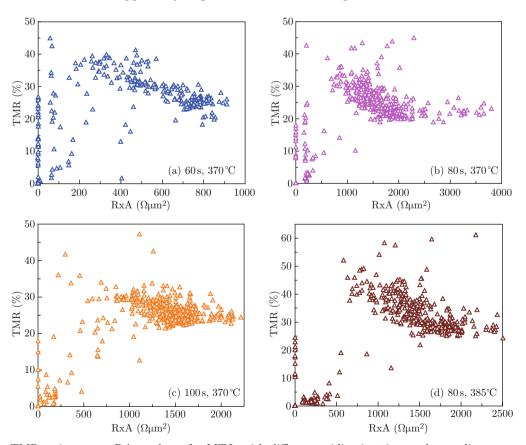
Fig. 2 TMR ratios versus RA products for MTJs with different oxidization time and annealing temperature.
