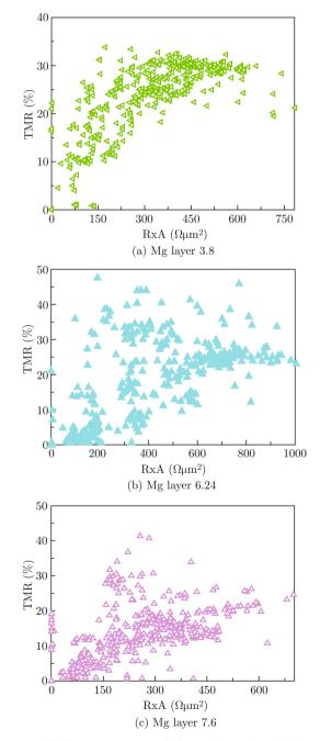
Fig. 1 TMR ratios versus RA products for MTJs with different Mg layer thickness.
