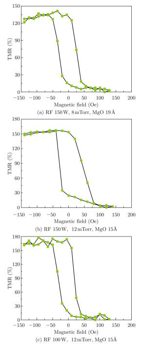
Fig. 4  $\,$  TMR curves of MgO barriers deposited with different deposition parameters.
