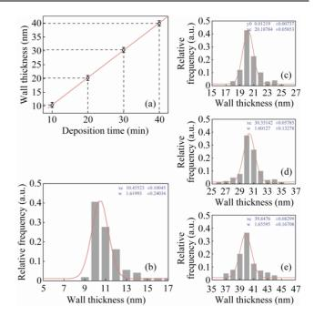
FIG. 2. (a) Deposition time vs. wall thickness plot. (b) Gaussian distribution of 10 nm wall thickness TNTs. (c-e) Gaussian distribution of 20, 30 and 40 nm wall thickness TNTs.
