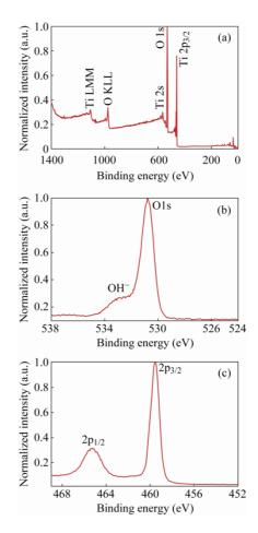
FIG. 4. XPS spectra of the synthesized TNTs (a) full range survey spectrum, (b) O 1s spectrum, (c) Ti  $2p_{3/2}$  spectrum.
