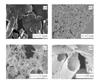
FIG. 1. (a) SEM image of the removed  $TiO_2$  layer from the template surface. (b) - (d) SEM image of bulk TNTs unhinged from polycarbonate template.
