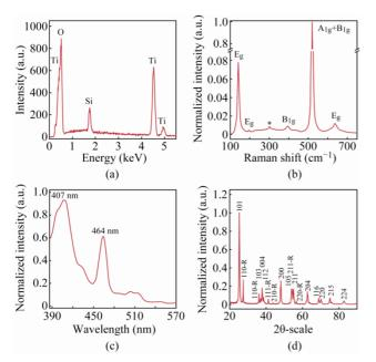
FIG. 3. (a) EDX spectrum of titanium dioxide nanotubes dissected silicon waver. (b) Normalized Raman Scattering spectrum of the TNTs. (c) Normalized PL spectra of the TNTs excited at 310 nm. (d) XRD-pattern of the TNTs, rutile reflexes marked with hkl-R, anatase only hkl.
