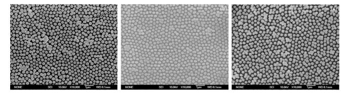
FIG. 4. SEM images of the PMMA nanopillar arrays obtained from the AAO anodized in phosphoric acid at an anodization voltage of 160 V at 2°C and the second anodization time of: (a) 2 min, (b) 5 min, and (c) 8 min.
