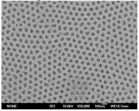
FIG. 6. SEM image of the imprinted regular  $TiO_2$  nano-pore arrays on a substrate by the as-fabricated PMMA/PDMS soft template as shown in Fig. 3(a).
