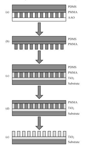
FIG. 1. Schematic diagram of the preparation procedures of the highly ordered  $TiO_2$  nano-pore arrays.
