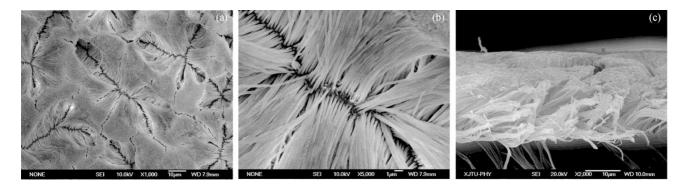
FIG. 3. Top view images of the PMMA nanowires obtained from the AAO template with the second anodization time of 4.5 h with a low magnification (a) and with a high magnification (b); (c) cross-sectional image of the PMMA nanowires.
