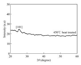
FIG. 7. XRD result of the imprinted  $\rm TiO_2$  nano-pore arrays after 450°C calcination for 30 min.
