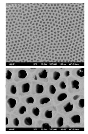
FIG. 2. SEM images of the AAO templates obtained: (a) in oxalic acid at an anodization voltage of 40 V at 5°C; (b) in phosphoric acid at an anodization voltage of 160 V at 2°C.
