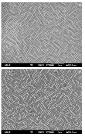
FIG. 5. SEM images of the PMMA nanopillar arrays fabricated (a) from the AAO template obtained in 0.3 M oxalic acid electrolyte at an anodization voltage of 40 V at 5°C; (b) surface morphology of the PMMA nanopillar arrays with some contamination.
