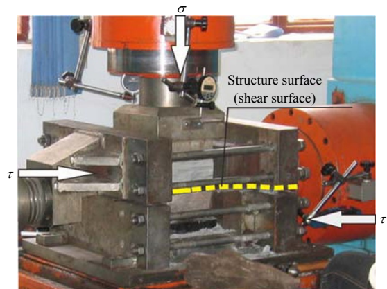
Fig. 7 Direct shear test apparatus for discontinuities
