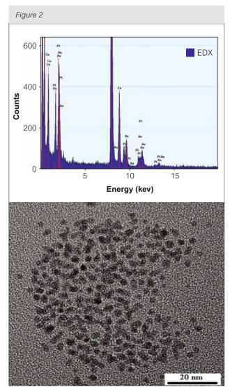
TEM micrograph and the corresponding EDX signal of Au/Pt particles obtained after total reduction (dose = 12 kGy) by electron beam irradiation of a solution containing [PtCl<sub>6</sub><sup>2-</sup>] =  $5 \times 10^4 \text{ mol.L}^{-1}$ , [AuCl<sub>4</sub><sup>-</sup>] =  $5 \times 10^4 \text{ mol.L}^{-1}$ , [PAA] = 0.1 mol.L<sup>-1</sup> and [2-propanol] = 0.1 mol.L<sup>-1</sup>
