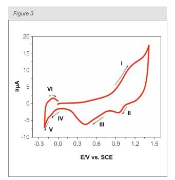
Cyclic voltammogram run in  $0.5 H_2SO_4$  with a glassy carbon electrode modified with electron beam synthesized Au-Pt alloyed NPs. The potential scan rate was 10 mV s<sup>-1</sup>. The reference electrode was a KCI-saturated calomel electrode (SCE) and the counter electrode a platinum gauze of large surface area. The solution was deoxygenated by pure argon
