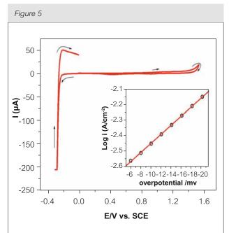
Cyclic voltammogram run in 0.5 M  $H_2SO_4$  (pH = 0.3) with a glassy carbon electrode modified by Au-Pt nanoparticles (50:50) in the absence of oxygen. The potential scan rate was 2 mV s<sup>-1</sup>. The reference electrode was a KCI saturated calomel electrode (SCE) and the counter electrode a platinum gauze of large surface area. Inset: Tafel analysis of the hydrogen evolution reaction
