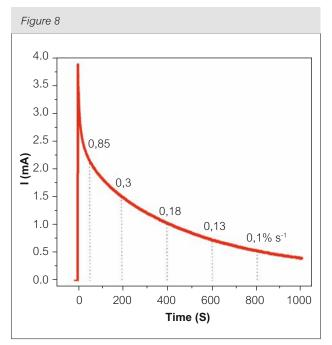
Chronoamperogram observed during the electrocatalytic oxidation of 1 M MeOH in 1 M KOH with an Au-Pt (50:50)-modified electrode. The solution was deoxygenated. The initial potential was fixed at – 0.55 V, stepped to 0.25 V and held there. The reference electrode was a Hg/HgO (1 M KOH) reference electrode and the counter electrode a platinum gauze of large surface area. The numbers on the curve indicate the current decrease percentage as a function of time
