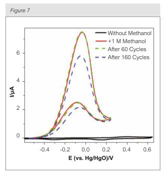
Comparison of the 1st, 60th and 160th cyclic voltammograms observed during the electrocatalytic oxidation of 1 M MeOH in 1 M KOH with an Au-Pt (50:50)-modified electrode. The solution was deoxygenated. The potential scan rate was 50 mV s<sup>-1</sup>. The reference electrode was a Hg/HgO (1 M KOH) reference electrode and the counter electrode a platinum gauze of large surface area
