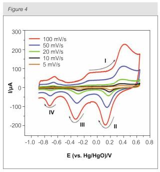
Cyclic voltammograms run in 1 M KOH with a glassy carbon electrode modified with electron beam synthesized Au-Pt alloyed NPs. The solution was deoxygenated by pure argon. The reference electrode was a Hg/HgO (1 M KOH) reference electrode and the counter electrode a platinum gauze of large surface area
