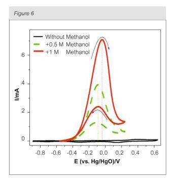
Cyclic voltammograms run with an Au-Pt (50:50)-modified electrode in 1 M KOH without MeOH ( — ) or containing 0.5 M MeOH ( – – – ) or 1 M MeOH ( — ). The solution was deoxygenated by argon bubbling. The potential scan rate was 50 mV s<sup>-1</sup>. The reference electrode was a Hg/HgO (1 M KOH) reference electrode and the counter electrode a platinum gauze of large surface area
