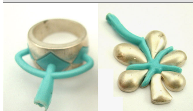
950 Pd casting with injected wax for the 2nd bi-metal casting process step; with kind permission of Vendorafa-Lombardi Srl, Valenza (Italy)
