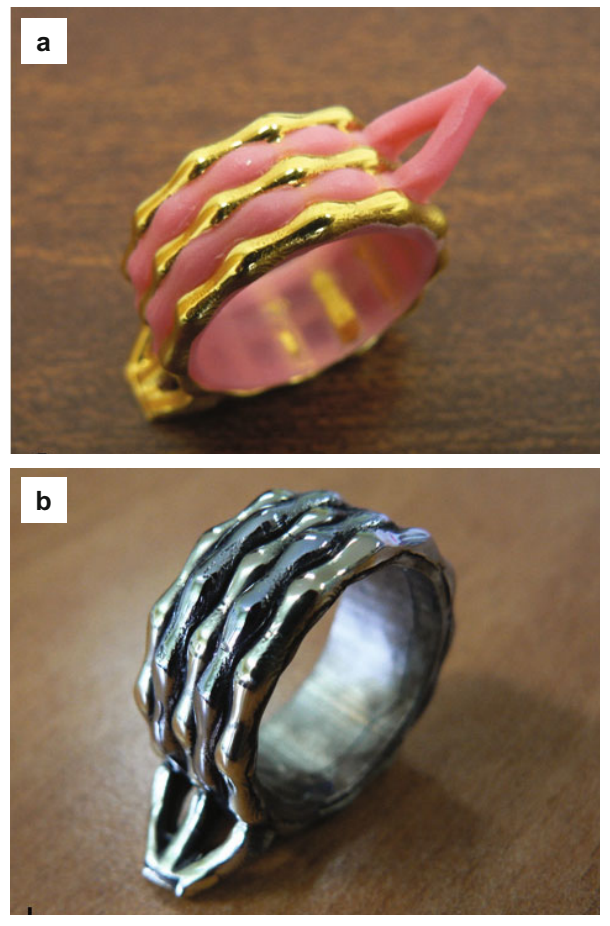
Bi-metal casting of a bi-color ring, microalloyed 14k blue + 14k green-yellow gold
