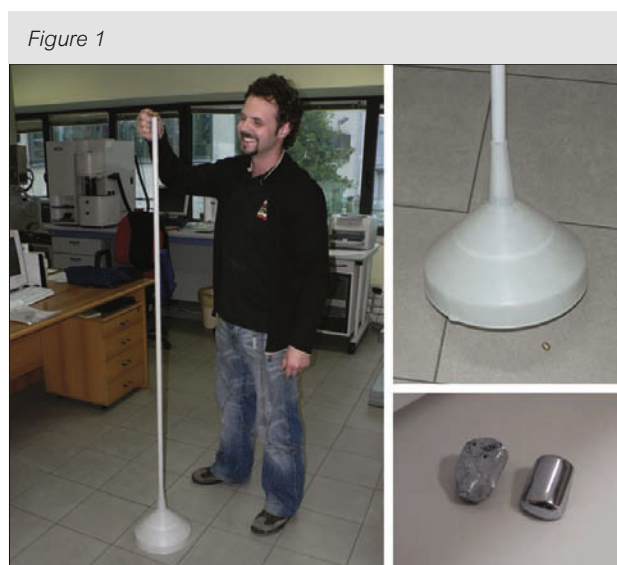
Figure 1 The 'crashmeter' for testing and quantifying the fracture resistance of blue and purple gold
