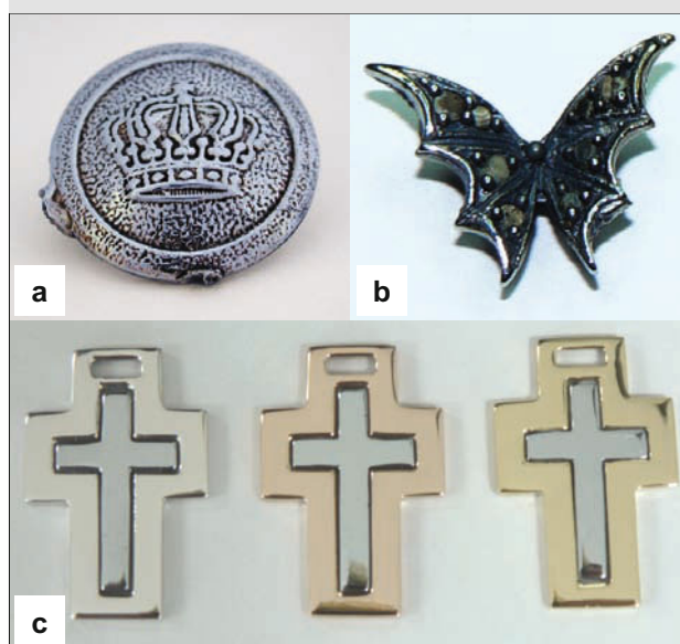
Castings of microalloyed 14k blue gold; a) and b) partial removal of the as-cast oxide layer; c) combination with standard white, yellow and red carat gold. Photo of the butterfly with kind permission of Co. Stephen Webster Ltd., London (UK)
