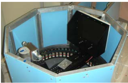
Figure 1. Working components in the Albion breast CT scanner.
