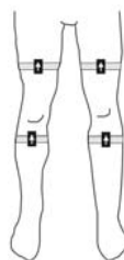
Figure 1. Experimental setup of four compact motion sensors strapped to the subject's thighs and shanks. The sensors provided absolute angular displacements in the sagittal plane, which was used as feedback information to modulate the stimulation sequences required to evoke gait.
