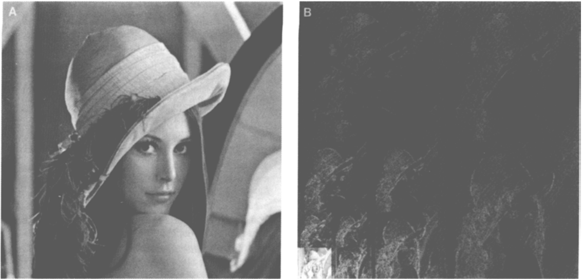
Fig 12. Wavelet compression. (A) The classic Lena image. (B) The subimages of the DWT for this image. Reprinted with permission from Manduca. 18
