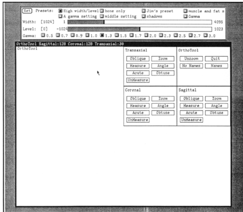
Fig 1. The user interface screen for OrthoTool. The controls in the upper right of the large window are used to manipulate the volume. The blank area around the controls is used for roving the cursor. The control window at top is used to manipulate window width and level.
