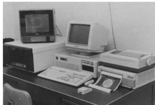
Fig 7. The PC-based imaging system. The tape read unit is seen at the left, while the video hard-copy unit is on the right.
